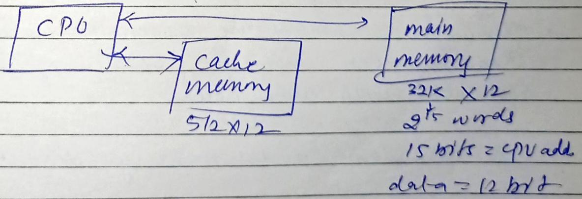
A cpu address of 15 bits is placed in the argument register and the associative memory is searched for a matching address.
